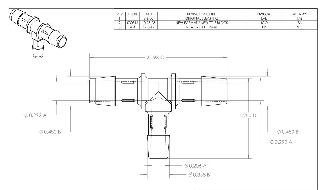
ANTI-ROTATION DEVICE 4 PLACES PER BARB NO MOLD PARTINGLINE PERMITED ON CONICAL SURFACES ALL DIMENSIONS TYPICAL MATERIAL-316SS VIEW SHOWN LOGO SIDE UP 'A' CAVITY DESIGNATED BY A SMALL DOT ON BARB NECK
